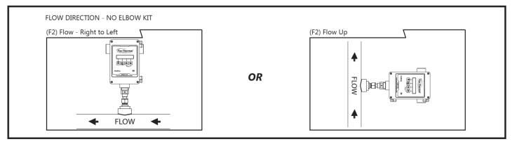
VERTICAL FLOW DIRECTION AND FLOWMETER POSITION
